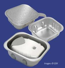
So the container manufacturer and its partners utilised their expertise in aluminium conversion technology and knowledge of the material's packaging attributes to create a durable, very high barrier container based on a deep draw aluminium tray, with a consumer friendly peelable lidding foil.
